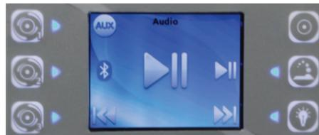
Using the upper control, press the “Mode” button TWICE in the bottom left hand corner of the screen to enter Audio Mode (if installed).
